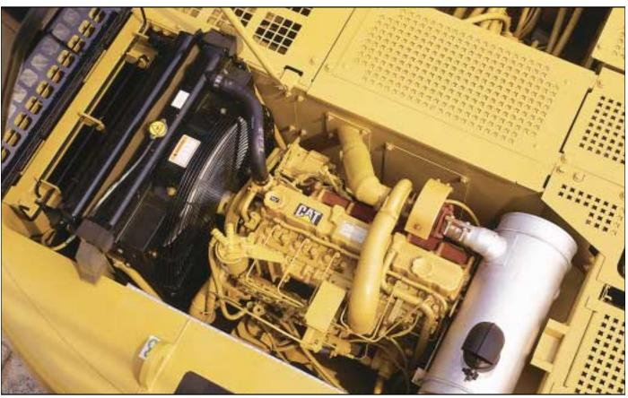
Automatic Engine Control with convenient one-touch command. Three-stage control maximizes fuel efficiency and reduces sound levels
