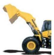
The long lift arms provide high dumping clearances and maximum dumping reach. The operator can even level loads on the body of a dump truck easily and efficiently.
