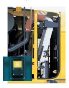
If the machine is operating in adverse conditions, the operator can reverse the hydraulic cooling fan from inside the cab by turning on a switch on the control panel. The coolers can also swing out for easy cleaning.
